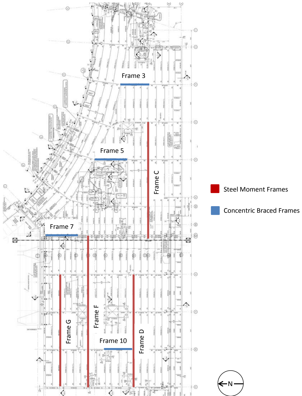
Figure 8 – Framing Plan (Courtesy of: Gannett Fleming)
